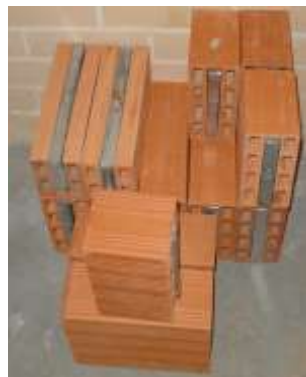
Fig. 11: Clay bricks with PCM macrocapsules[20] (which come in a variety of forms), and the heat transfer fluid
